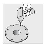
Unroll roofing membrane, mark and cut out centre hole Ø 200 mm.
