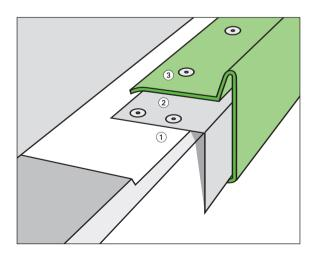
Rhepanol laminated metal sheets (de-burred cut edges) are applied with a clearance of 4 mm (profile length max. 2.00 m). With profile lengths exceeding 2.00 m, the joint clearance must be 10 mm.
