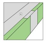
Welding the Rhepanol hg flashing strip to the roofing membrane with the handheld hot-air welder or the welding machine.
