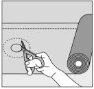
Weld the roofing membrane to the flange.
