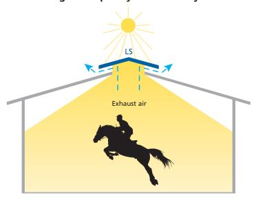
Sophisticated aerodynamics ensure high air exchange rates and the LS version ensures wide light dispersion avoiding cast shadow.
